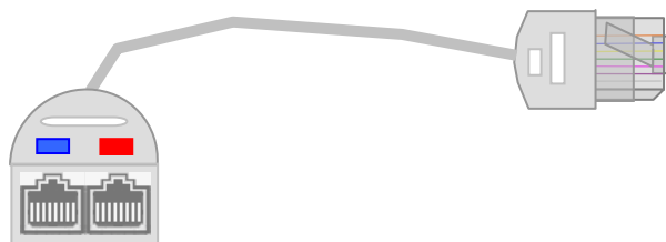
Figure 2-6 Two-way Hub for RJ48C/M
