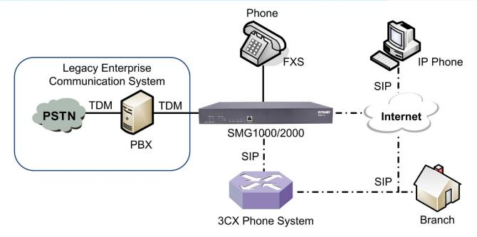
The introduction of SMG1000 Analog Gateway and 3CX Phone System ensure Qing Chun Bao to upgrade legacy communication system and realize new enterprise communication infrastructure and be capable of free switch between PSTN and IP network environments. The capabilities of the new solution includes:
