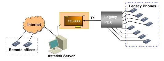
Figure 1-3 Application Model I: Traditional Telephony System
