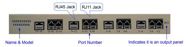
The four pins (no polarity) in each RJ11 jack connect to two phone lines: the middle two pins of each RJ11 correspond to an odd-numbered port (e.g. the  $1^{st}$ ,  $3^{rd}$ ,  $5^{th}$ ,  $7^{th}$ ... port), and the outer two pins to an even-numbered port (e.g. the  $2^{nd}$ ,  $4^{th}$ ,  $6^{th}$ ,  $8^{th}$ ... port). When linking this box to the SHT -4/8B voice boards, all you need to do is use RJ11 heads with similar arrangement in their 4 pins.
