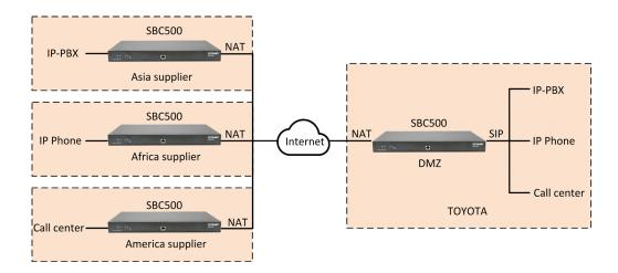
Synway SBC500, an organic component of communication solution, often is implemented as connection point between internal and external networks, being used for bridging IP-based multimedia transmission among different IP networks and ensuring high level of communication security in diverse networks of enterprises, services providers and carriers.
