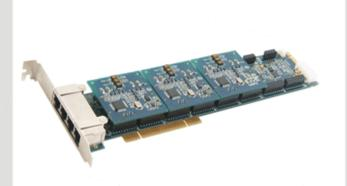
To configure any density (2~16 channels), the BRI baseboard can be mounted on a backplane, which has dual-bus-connectors to mount additional daughterboard for higher density. For that, a BRI baseboard and its daughterboard share the synchronous clocking of the BRI baseboard's PCI/PCIe interface. This add-ons architecture(BRI series) is powered internally.
