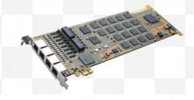
IP & TDM boards consist of three product lines: SHN series for IP network, SHD series for E1/T1/J1 digital network, and SHT series with analog interface. Besides a complete range of media resources, such as fax, conferencing, compression, echo cancellation for voice enhancement, they also combine various built-in signaling protocol software packets, which include SIP, H.323, SS7 (MAP/SCCP/ISUP/TCAP/TUP/MTP1~3), ISDN variants, CAS and more
