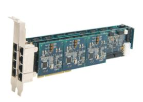
Each BRI baseboard or its daughterboard has four sockets to mount four S/T BRI modules. One S/T BRI module has two S/T four-wire interfaces, which supports TE or NT mode. 1~8 S/T BRI modules can be installed in BRI's baseboard/daughterboard(connected by a backplane) for a total 16 ISDN BRI lines
