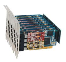
To configure any density (2~32 channels), the FXM baseboard can be mounted on a backplane, which has up to eight bus connectors to mount additional daughterboard for higher density. For that, a FXM baseboard and up to seven daughterboards (with no PCI/PCIe form factor) can be combined together by this backplane, and share the synchronous clocking of the FXM320X baseboard's PCI interface. This add-ons architecture(FXM series) is powered internally.
